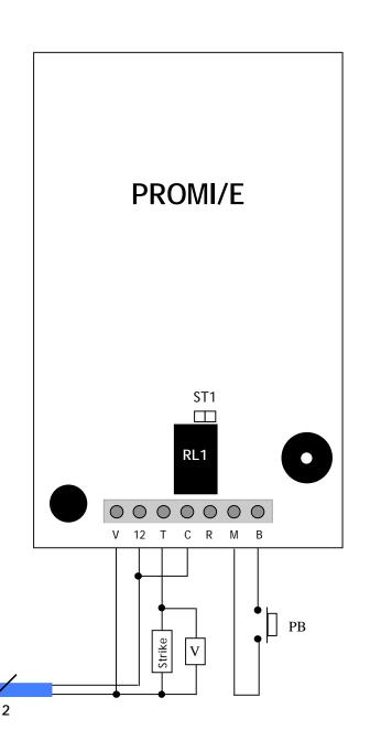
Do not forget to put the varistor on the lock.
