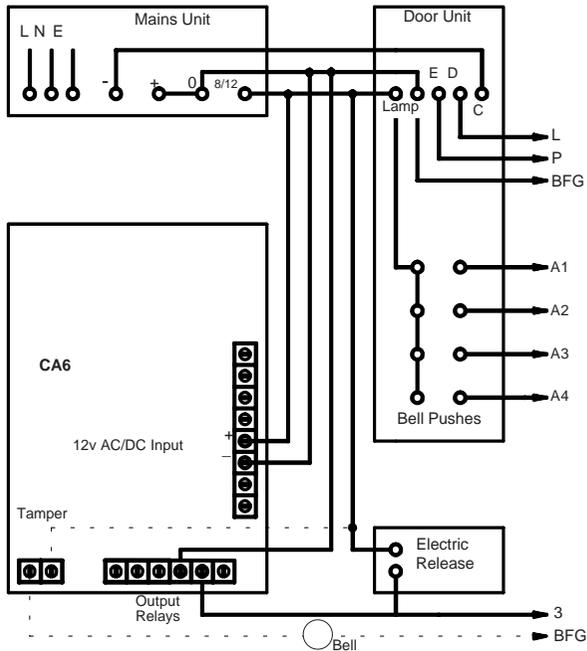
The CA6 shown above connected with Entryphone® plan 1. The tamper connections are optional. The second relay is shown not used.
