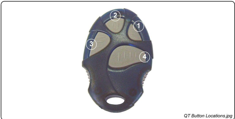
Figure 1: Button Configuration for the ImproX (QT) Quad Transmitter Programmed in “Dynamic Code Transmission Mode”
