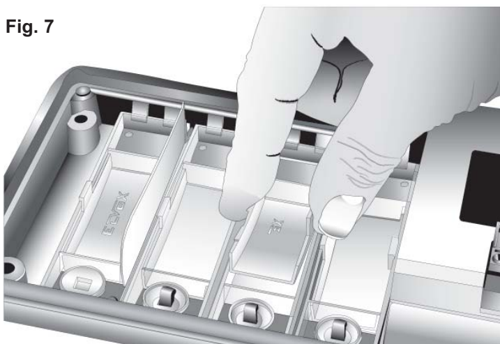
Fig. 7 - Press gently on the module with push-buttons to remove the name-tag holder.
