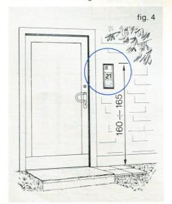
art. 2147 camera module with an illuminating light, heating resistance and thermostat for limiting the maximum temperature. Power is supplied to the system at 24 volts by means of the transformer Art. 45.14. All electrical functions which are common to the basic installation (timing, signals, etc.) are all obtained from the electronic power supply unit Art. PS010.
